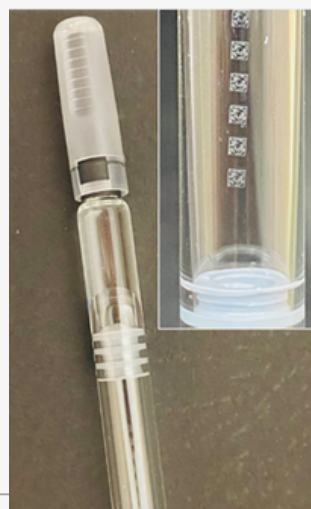
Figure 4: Marking on single use syringes glass body : 1,5mm DM 14x14 datamatrix code is marked in <50ms, using NIR ultra-short pulse laser. Multibeam marking reduces significantly the risk of micro-cracking.
