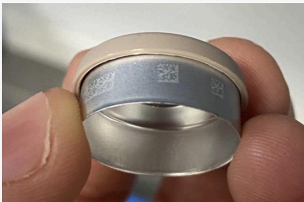
→ Figure 5: Marking on vials anodized aluminium caps: 2mm DM 12x12 datamatrix code is marked in one single pulse (marking time <10ns), using NIR pulsed laser
