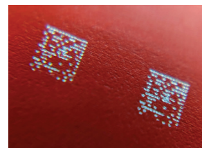
Beverage Wine caps, coated aluminium Discrete traceability Marking time <10 ns (one pulse)
