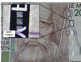
Bank Bank note, Metalized PET Roll-to-roll processing Anticounterfeiting 2000 codes per second
