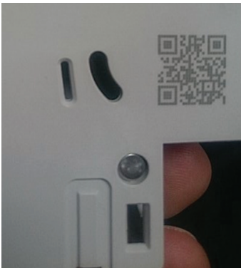
Consumer goods / Fuse breaker - PA66 Secured traceability / Marking time: QR code 250ms / Seal Vector 750ms
